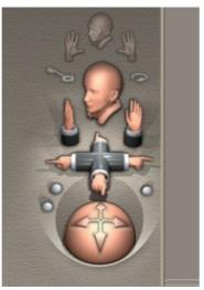
To change the layout of the screen, use the viewport selector at the bottom of the preview window. This enables you to arrange a number of different views on the screen at the same time so that you can see how an item looks, say, from above and from the left side at the same time.
